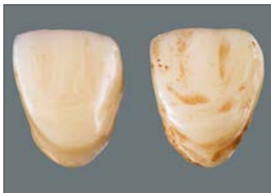
Photo 1: to the left: completely polymerized, hardly any discoloration to the right: incompletely polymerized; strong discolorations
