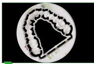
Bridges with skeletonized sinter support following the milling process.
