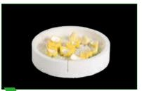
Manually precolored restorations in the sintering dish MS, ready for speed sintering
